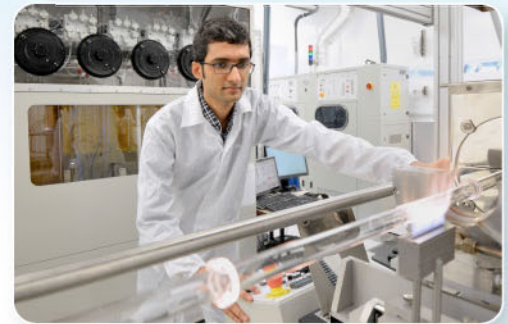
Dr Sidharthan Raghuraman works on the Modified Chemical Vapour Deposition (MCVD) system, which is used for the fabrication of optical fibre preforms.
