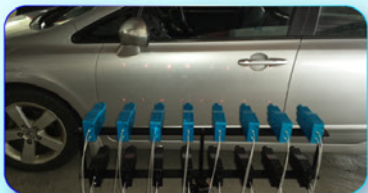
Multi-point Laser Doppler Vibrometer for Car Body Vibration Measurement
