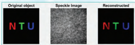
Using only simple optic elements and speckle patterns, Asst Prof Cuong is able to capture sharp, multi-coloured images without lenses, colour filters or expensive photodetectors.
