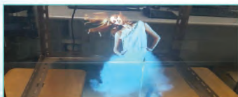
By placing a projection film over a transparent glass panel, Assoc Prof Chen's technology makes it possible to project images such as the dancer shown here, onto the glass, while the audience can also see through the projected images.
